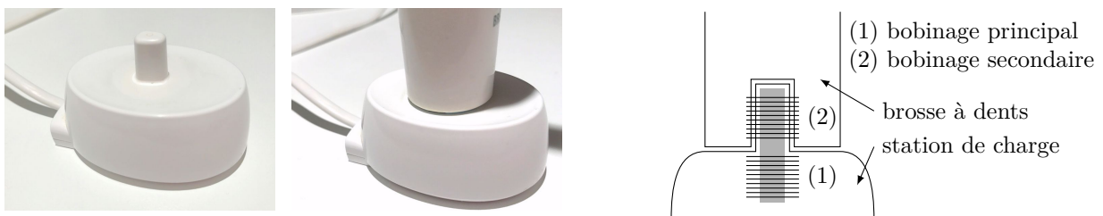
Figure 9 Station de charge
